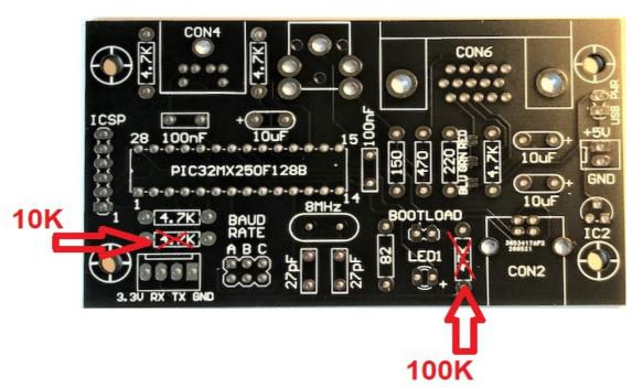
On the PCB there are two resistor values wrong, just place the right resistors on the indicated place as indicated by the red arrows. The building kit contains the right resistor values.
