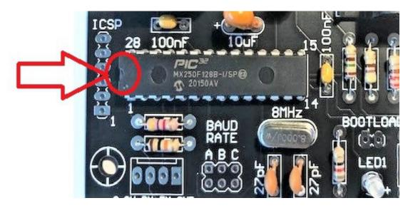
Look twice to make sure the microcontroller is facing the right way before you solder it. because it is very difficult to take it out again after you soldered it in. Short soldering and not to hot.
