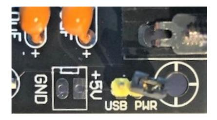
The jumper on the USB PWR connector is only placed on both pins if you connect the module to the USB connector. It will get its power supply from the USB in that case. If this is NOT the case do NOT CONNECT this header. Never connect the USB header and also the 5 volts power supply. Just choose for one of the two.
