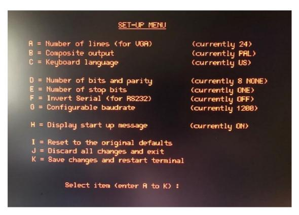
Here you can make all the needed changes and save them, by pressing K. Option G is for changing the baudrate. If the standard is 1200 you can change the baudrate with the jumpers on the PCB. But this is not really needed normally. So just use the setup here. If you save the changes the module will remember them after powering down and up again.
