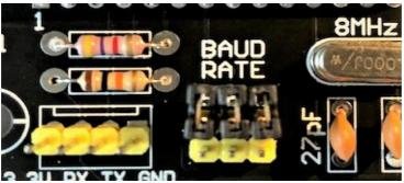
The baudrate jumpers are not really needed because you can also set the baudrate in the software, later more about this. On the picture they are placed on just one of the pins in the neutral position. In the other downloadable manual you can see how to set the baudrate with the jumpers. Headers for ICSP and bootload are not needed. You can also place a header on the 5 volts input but maybe you wnt to connect this in another way.
